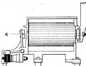
Fig. 5.—Clutch Magnet of Signal Motor.
