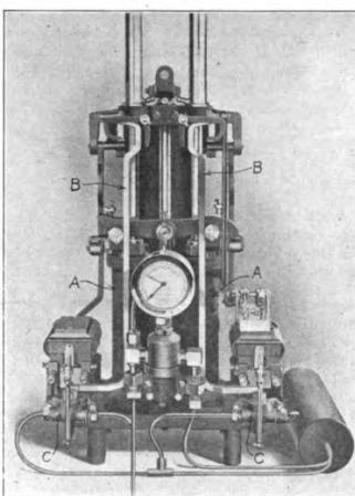
Fig. 1.—Electro-Gas Signal Apparatus.
