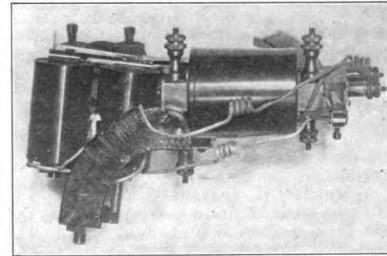
Fig. 3.—Signal Magnet and Hold-Clear Magnet—Old Style.
