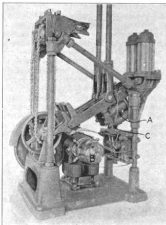
Fig. 4.—Electric Motor for Semaphore Signal.
