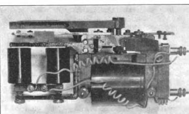
Fig. 6.—Signal Magnet and Hold-Clear Magnet—New Style (Top View Looking Down).
