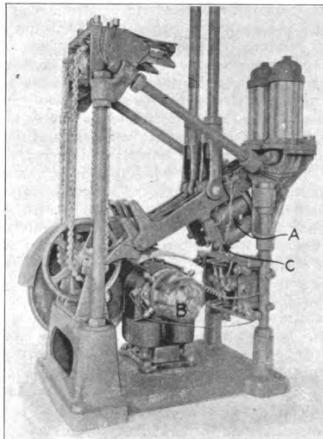
Fig. 4.—Electric Motor for Semaphore Signal.
