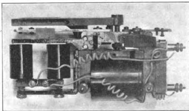
Fig. 6.—Signal Magnet and Hold-Clear Magnet—New Style (Top View Looking Down).
