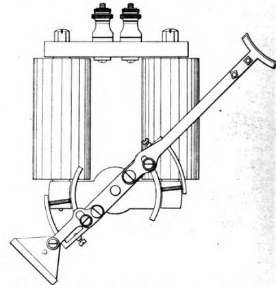
Fig. 2.—Signal Magnet for Enclosed Disk Signal.
