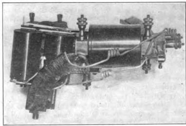
Fig. 3.—Signal Magnet and Hold-Clear Magnet—Old Style.
