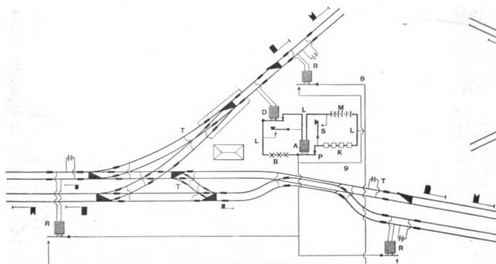
Fig. 1. Automatic Electric Locks for Switch Levers; Diagrams of Connections.
