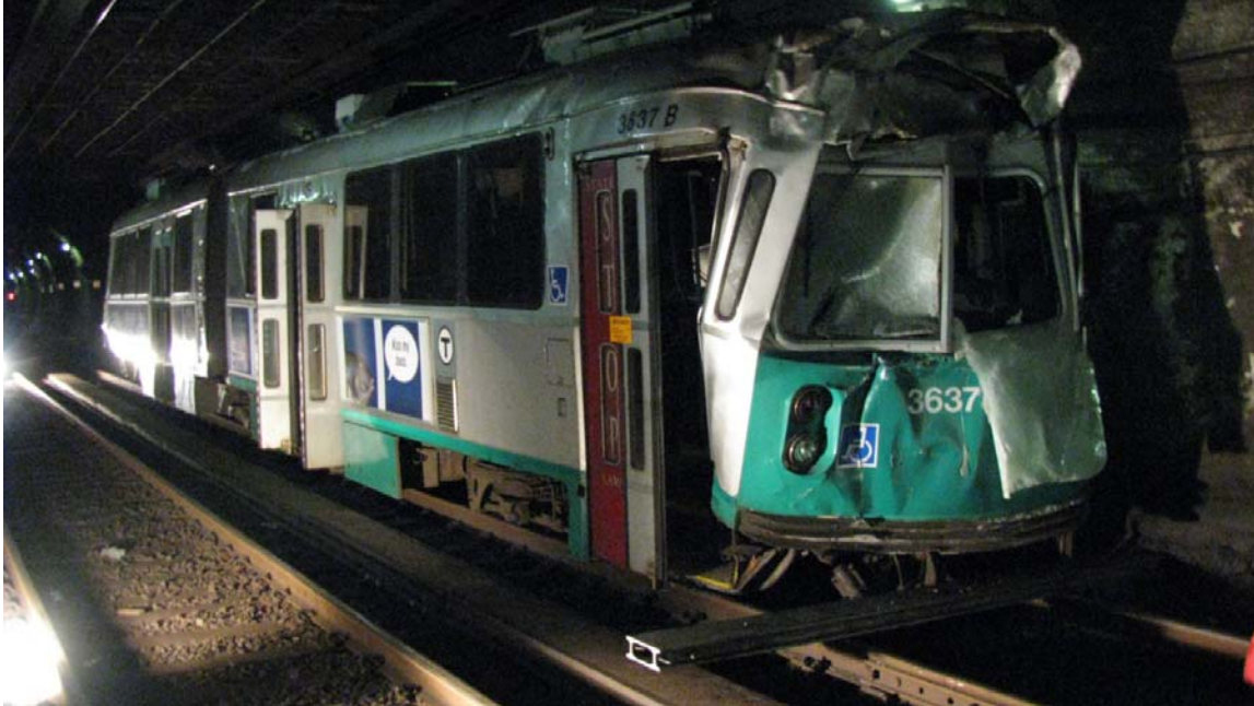
Figure 3. Photograph showing damage to rear of standing train 3808.
