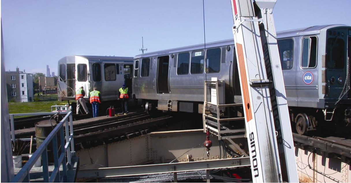
Figure 1. Derailed lead cars of train 003.
