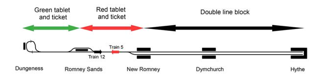
Diagram of running lines and methods of working on the Romney, Hythe & Dymchurch Railway. Station details and minor stops omitted
