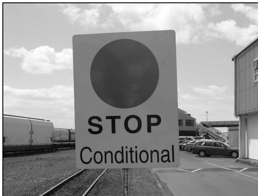
Figure 3 Conditional Stop Board
