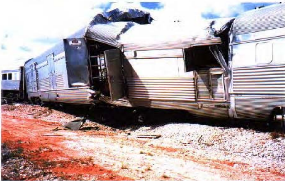
Figure 4: Damage to IP Coach HM311
