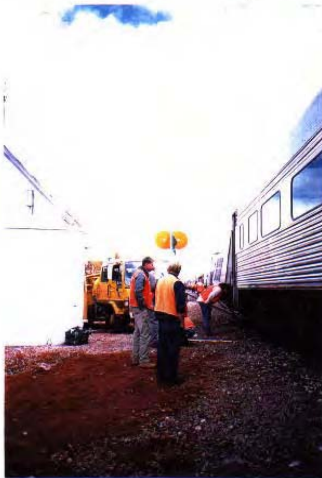
Figure 9: Flashing light indicator and yellow dumb bell showing points set for loop.
