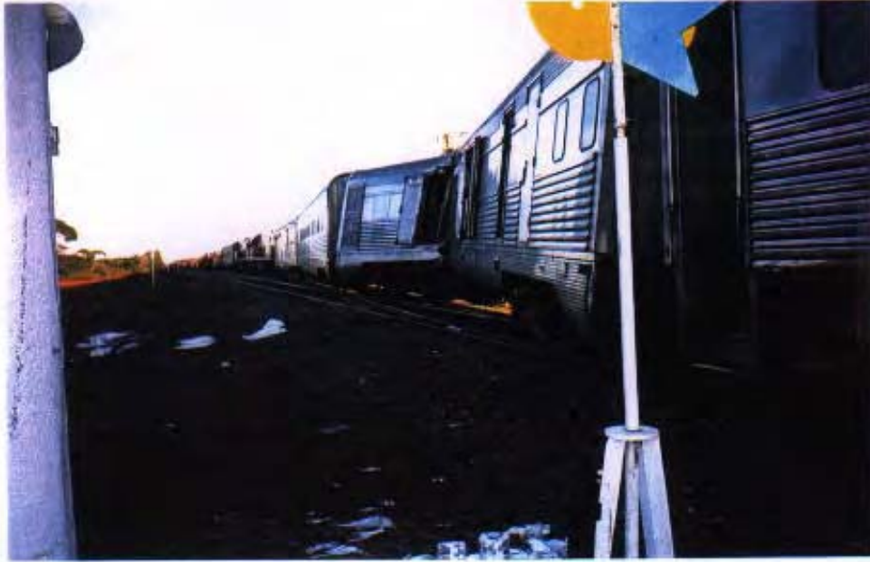
Figure 5: Damage to IP Coach HM311 positioned on turnout.
