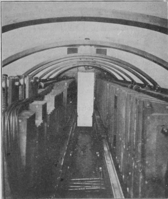
Interior of No. 2 Apparatus Cab of the General Electric Locomotive with Roof Removed
