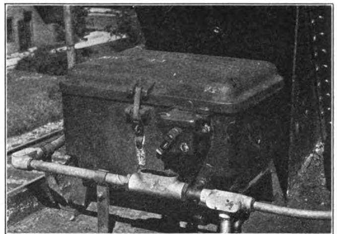
Relays and Timing Element Are Housed in a Cast-Iron Box on the Tender
